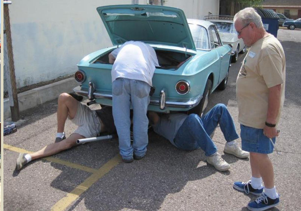
Above: Quick-change of a throwout bearing on Dave Whitaker's Pacific 1964.
