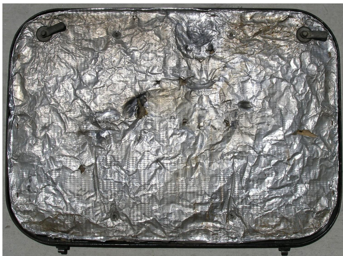
Original engine trapdoor insulation (above) Stripped engine trapdoor (below)
